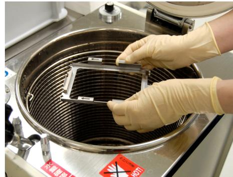
Sterilizing the holder with an autoclave
