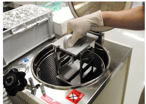
**Sterilizing the carrier with an autoclave**
