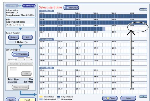
The figure on the right shows an example of multiple scheduled observations set at 6 hours intervals from 17:00. To set 55 minutes for the scheduled observation time, press the period of 17:00. The one hour period from 17:00 is displayed in yellow.
